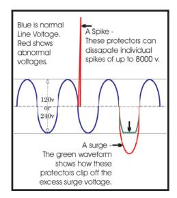
The VZPRO and X13PR protectors are *plug-in* devices - external to the motors - that intercept most voltage problems **BEFORE** they get a chance to do any damage to the motor or module. The chart at left shows what AC waveforms look like on an oscilloscope, and also shows what some damaging transients might look like.
